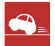
(3) Deceleration alarm screen: The screen will appear when ECO STAR detects hard braking; red LED will light on and beep to warn the driver. Alarm will be continued until deceleration is improved.
